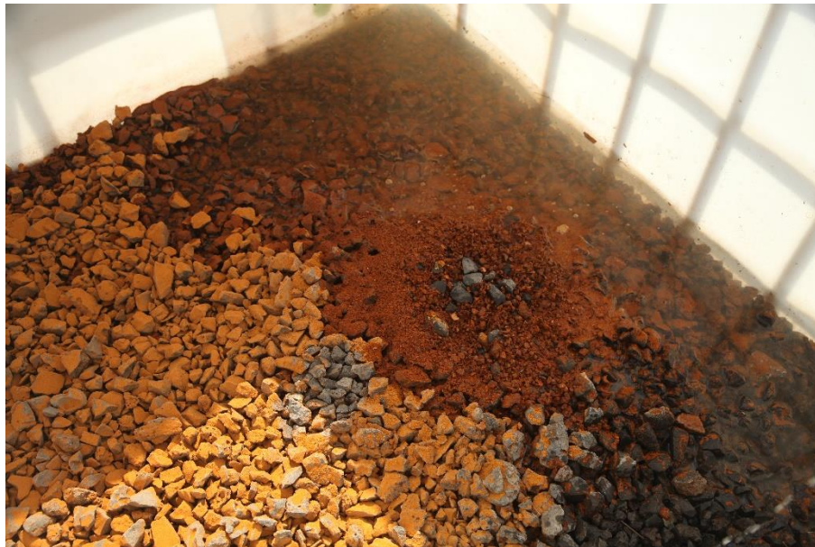
Figure 7. Sludge formation on top of the inert slag substrate of the VFR at the FND site
