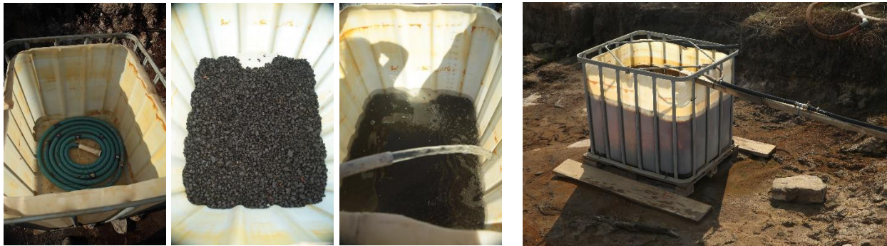
Figure 4. Setup of the VFR in a 1 m 3 IBC. From left to right: spiral-laid vacuum hose, 15 cm high slag layer, filling of the VFR with AMD, field trial VFR in operation
